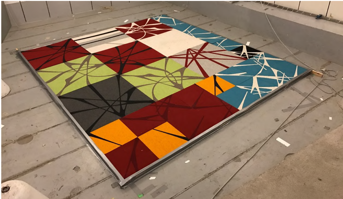
Photo of 15 mm Fraster Twister Plus acoustic panels with mounting depth 45 mm in the reverberation room.
