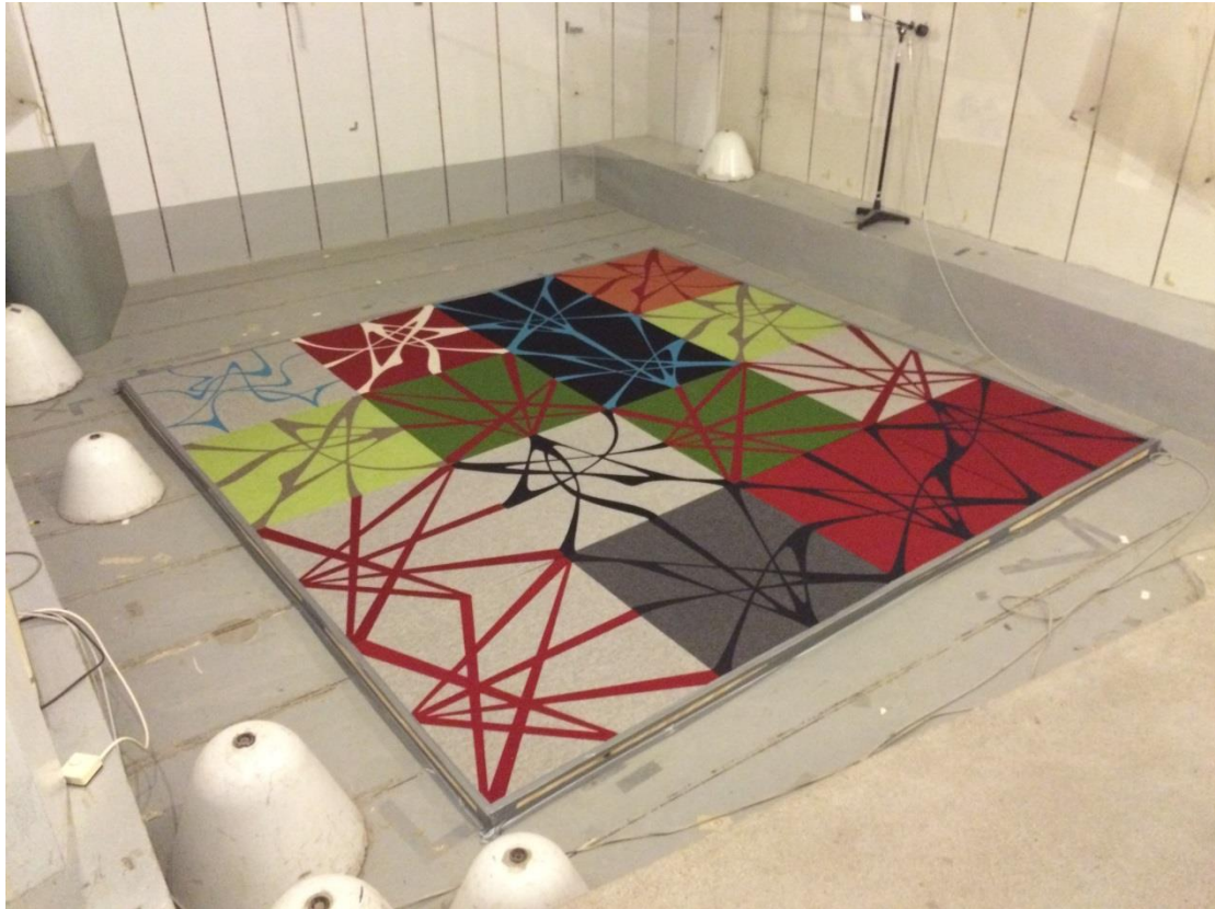
Photo of 15 mm Fraster felt Plus acoustic panels with mounting depth 65 mm in the reverberation room.
